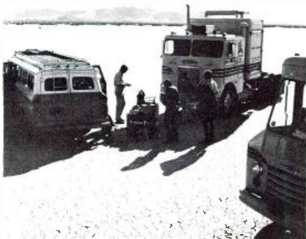
Figure 5. The proper solution was to record the audio in the bus shown at the left, after it was moved away from the generator truck seen at center. The t.v. truck just poking into the picture at the right was used as a control room where both picture and sound were laid onto video tape.
